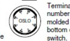
Terminal numbers molded on bottom of switch.
